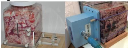
A 1.9 GHz half wavelength ( $\lambda/2$ ) dipole antenna (left) and a 1.9 GHz rectangular waveguide (WR-430) RF source (right) placed against the ex vivo bovine brain tissue in the cubical plastic containers.
