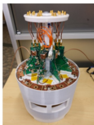
Figure 3. Constructed head coil exposing RF front end electronics including eight circuit boards, each with transmit-receive switch and preamp, or alternatively with CMOS circulators and preamps for STAR operation.
