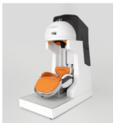
Figure 1. Head-only, 1.5T MRI system. Features include YBCO HTSC cryo plate cooled asymmetric magnet, multi-coil field encoding/shimming, 8-channel FPGA controller, non-uniform field imaging, and our eight-channel TR+STAR coil featured here.
